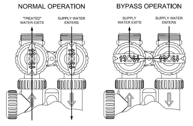
During Normal Operation, the arrows on the bypass valves should be pointing in the direction as the flow of water in and out of the system.
