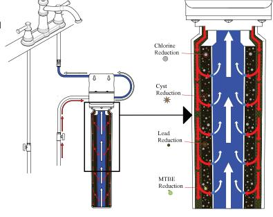
System tested and certified IAPMO against NSF/ANSI Standard 42, 53 & 401 for the reduction of the claims specified on the Performance Data Sheet
